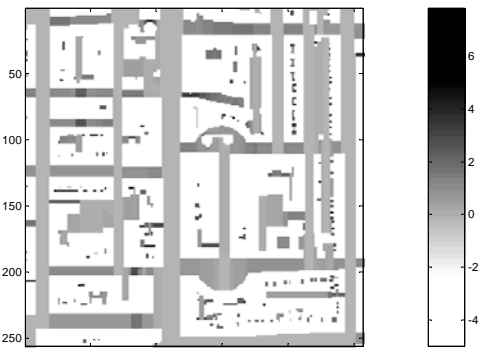
Figure 3 - Height to width ratio in the North/South (azimuth=0) direction on the DEM; values in the streets range between 0 and 7
