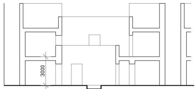
Fig. 11. Diagrammatic section of the selected base case courtyard. Dimensions based on Morris [13] and Talib [14].
