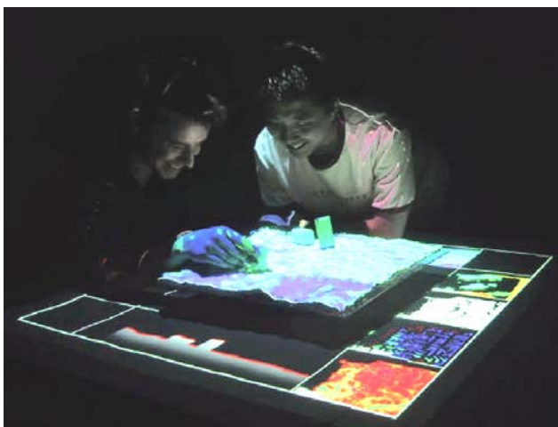
Fig 1 Illuminating Clay in use — digitally augmented clay model of landscape provides the input/output for GIS (Geographic Information System) simulations.
