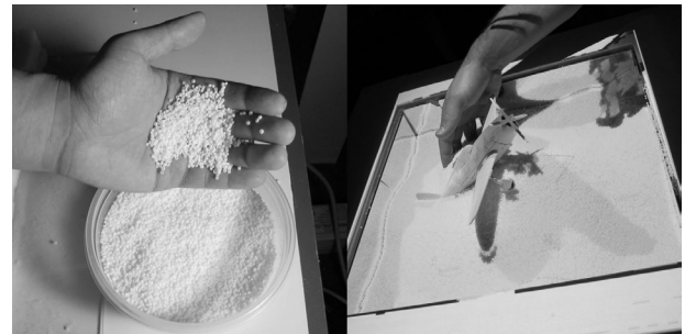
Figure 4. Glass beads to explore a cross-section of a CFD simulation of air temperature around an airplane fuselage
