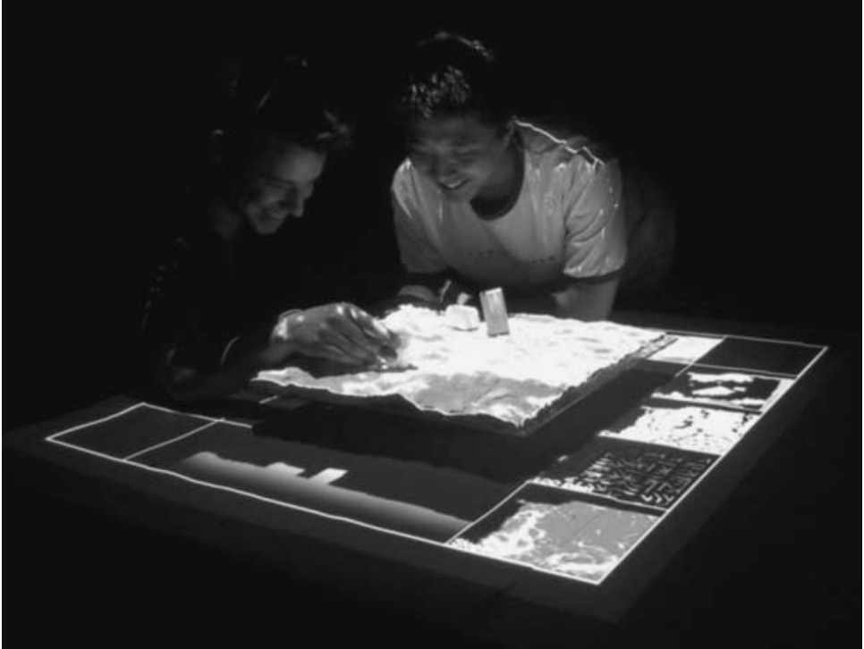
Figure 1 Illuminating Clay : A landscape model made of clay provides the input/output for GIS simulations
