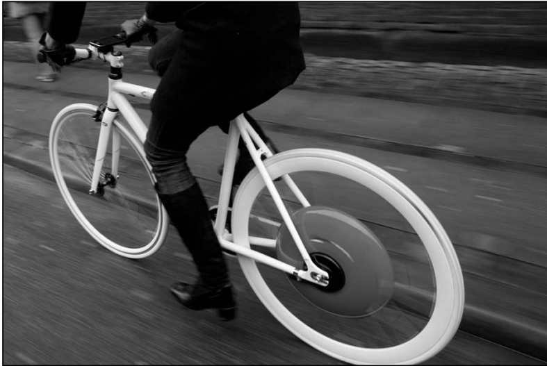
Figure 5. Copenhagen Wheel retrofitting a conventional bicycle, MIT SENSEable City Lab©
