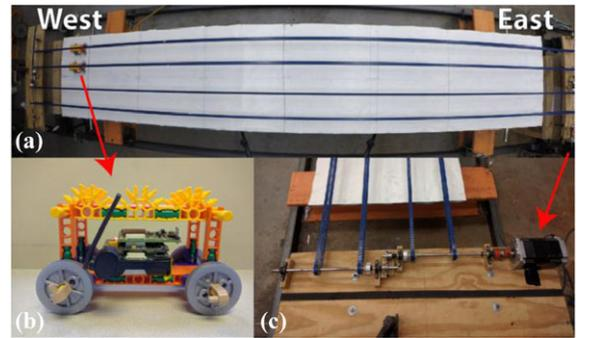
**Fig. 4.** (a) Aerial photo of beam specimen at Lehigh University. Two mobile sensor cars are shown at their starting positions; (b) mobile sensor car equipped with a wireless accelerometer; (c) step motor, shaft assemblage, and four belts.
