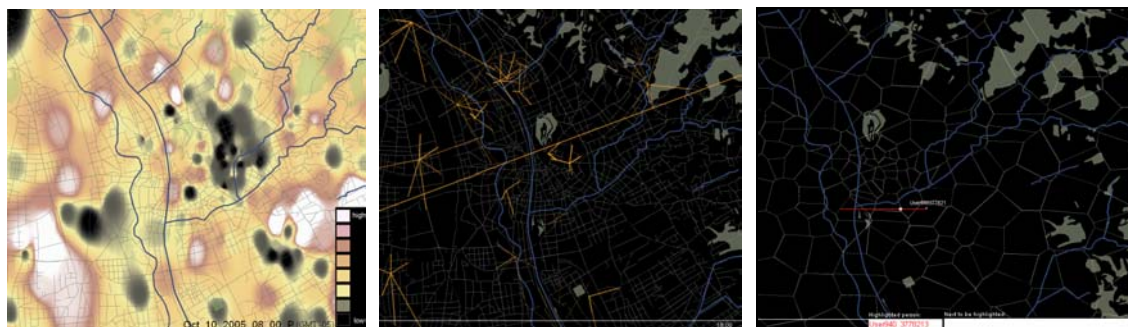
Figure 3: From left to right: visualization of cellphone traffic intensity on 10 October 2005 at 8 pm; visualization of traffic migration (handovers) at the same time; traces of registered users at the same time. During the exhibition period these maps can be seen in real time at the URL: http://senseable.mit.edu/grazrealtime
