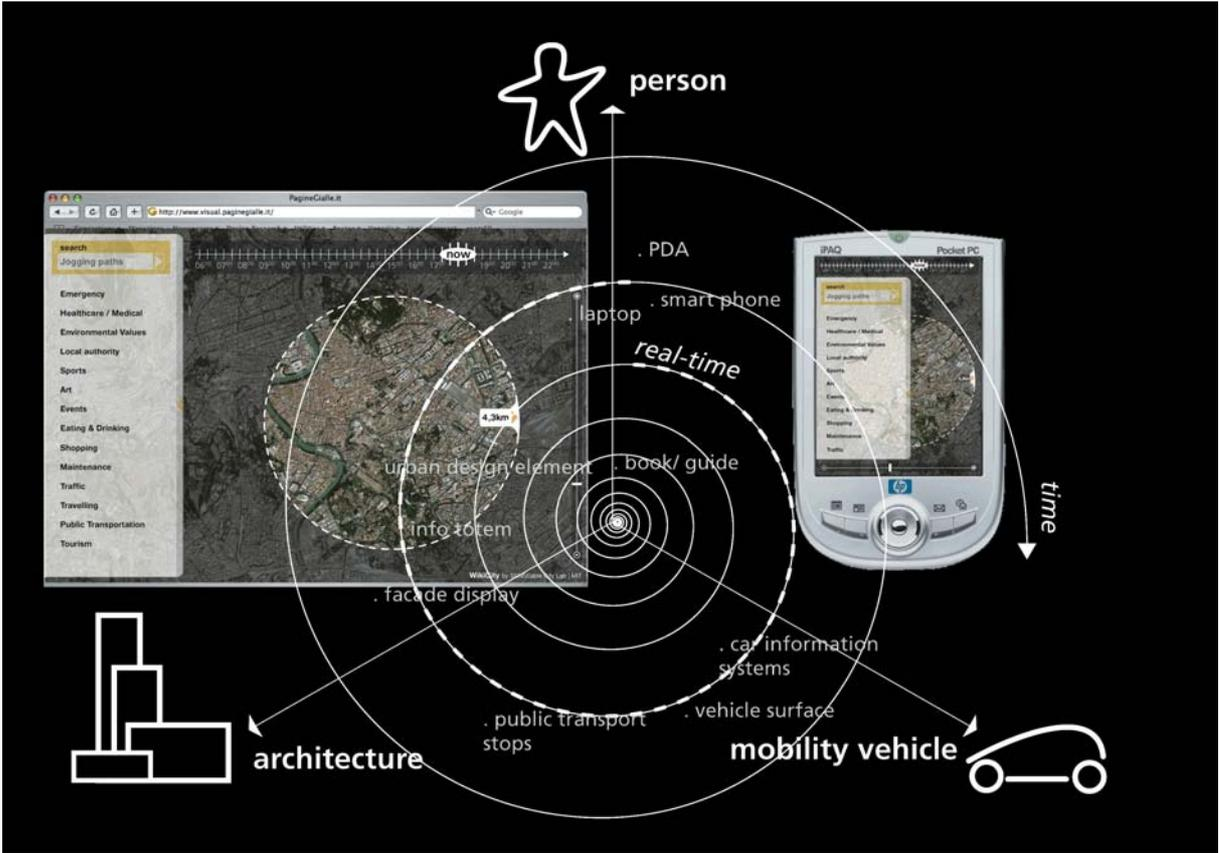
Figure 1. Device Interface study. WikiCity explores different interface modalities that create connections between the virtual data and the actual physical world where these data is accessed by users. Interfaces to WikiCity can be more closely positioned to the built environment, to moving vehicles or to the user. Functional elements of the 2D display interface include: search field, "local" distance range indicator, time range indicator and a results area.
