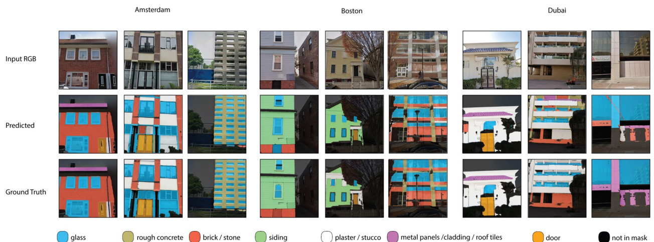
Fig. 3. Example output segmentations on panoramas in Amsterdam, Boston, and Dubai across diverse material types.
