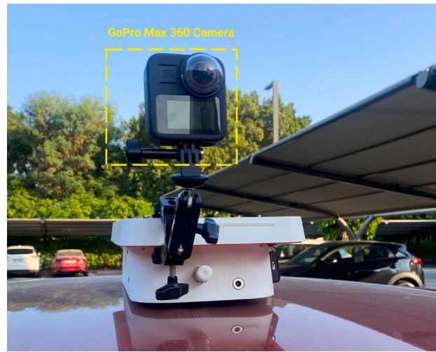
Fig. A.1. Platform setup for street view image collection: a GoPro MAX camera mounted on a vehicle, enabling panoramic data capture along the surveyed routes.
