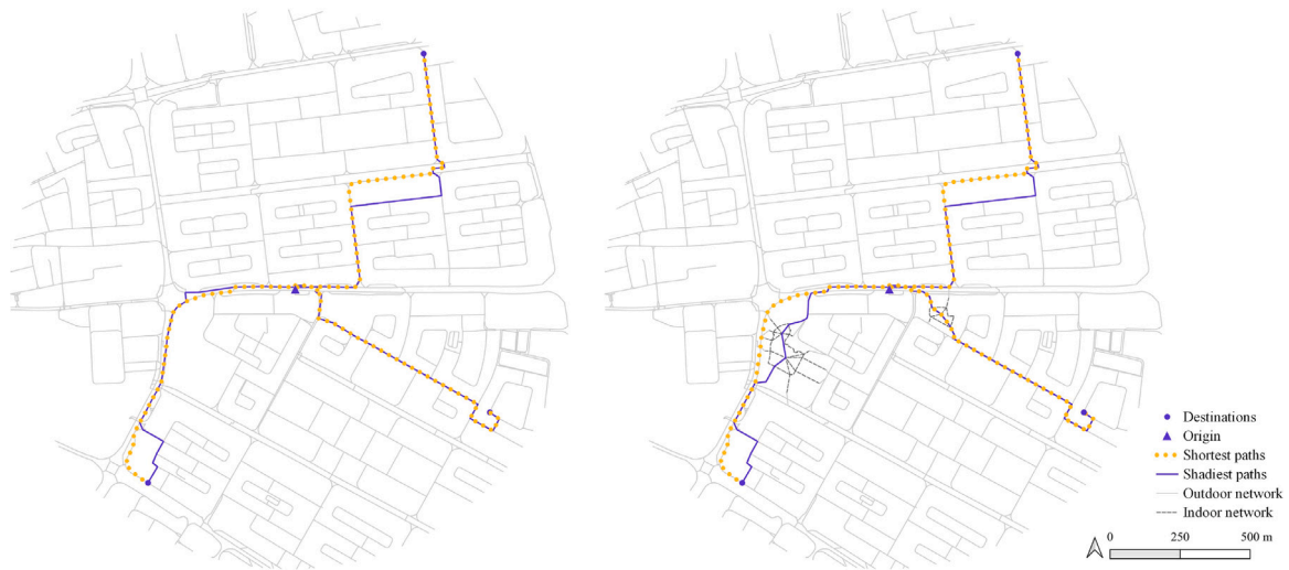
Fig. 11. Three representative pairs comparing the shortest path vs. the optimal shadiest path during 8:00–9:00 AM on 21st December at Salah Al Din metro station. The left map shows routes calculated using the outdoor network only, while the right map incorporates the combined outdoor-indoor network, illustrating differences in pedestrian route choices when indoor pathways are included.
