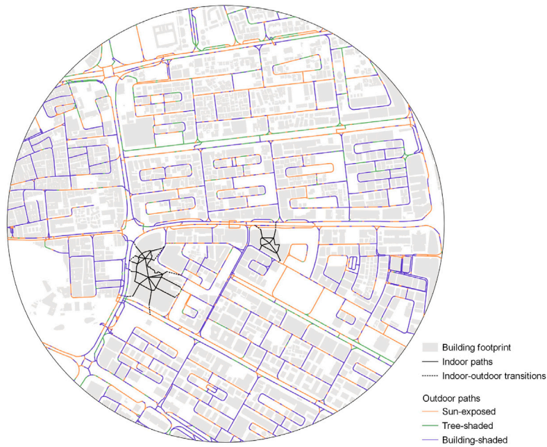
Fig. A.5. Shade conditions between 8:00–9:00 AM on 21 December at Salah Al Din station, showing building footprints, indoor paths, outdoor paths (sun-exposed, tree-shaded, and building-shaded), and indoor–outdoor transitions.
