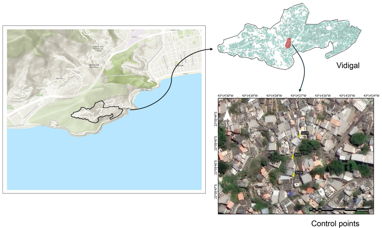
Fig. 8 | Scanned location and control points in Vidigal. Three control points were labeled as yellow before the LiDAR scanning, shown in the bottom right corner.
